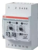
The RD3 family of electronic residual current relays provides residual current protection and monitoring functions according to IEC/EN 60947-2:2006 annex M and can be used in conjunction with all S 200 automatic devices and Tmax range moulded case devices up to T5, for industrial installations.
